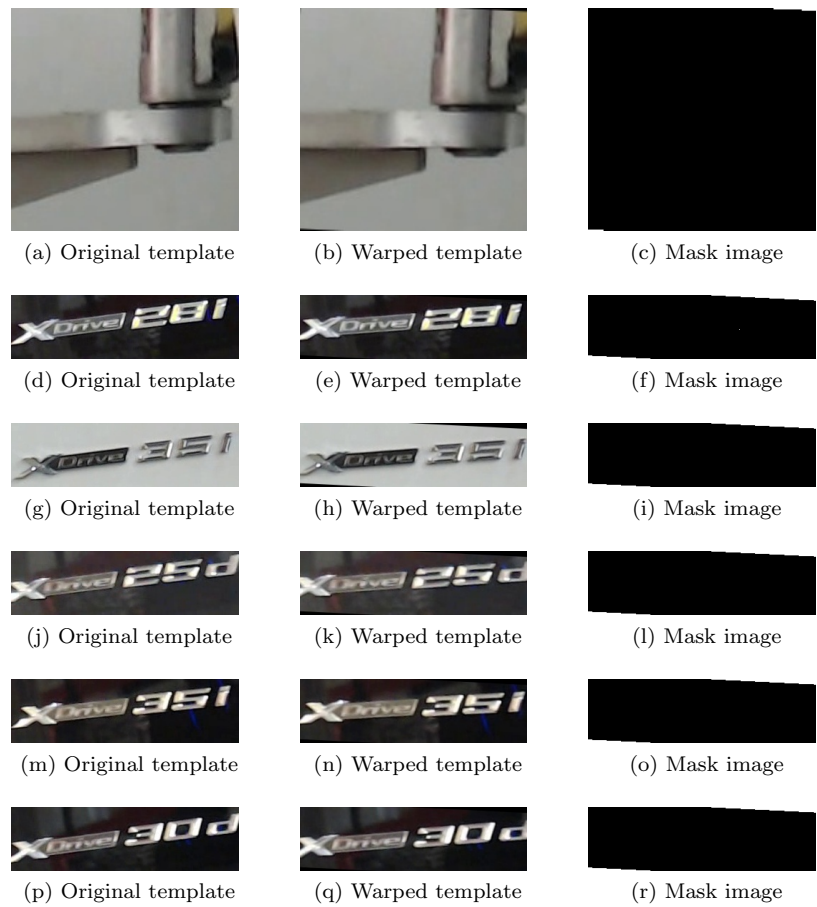
Figure 3.23: The effect of applying the affine transformation found in figure 3.19 on template images of the door line the BMW plant.
