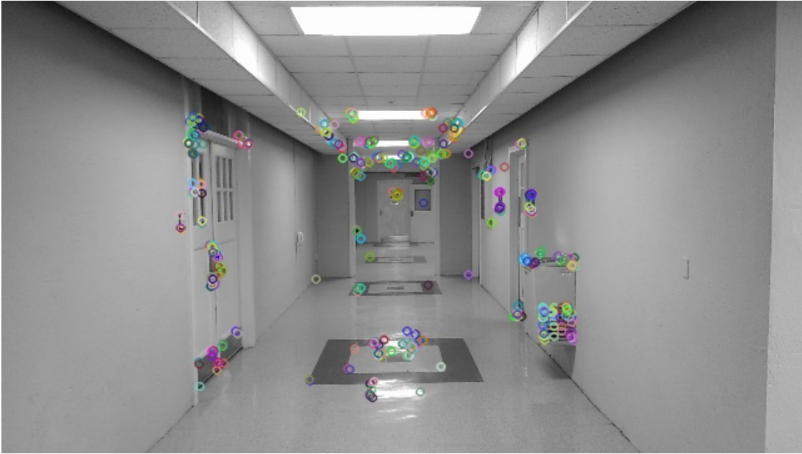
Figure 3.13: ORB keypoints detected in the after-bump image.
