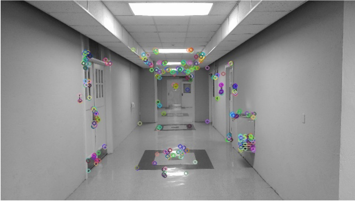
Figure 3.12: ORB keypoints detected in the before-bump image.
