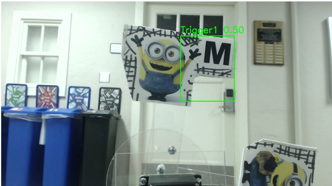
Figure 3.27: A screen grab of the setup program running the post-bump video with the original templates of the simulation testbed. The trigger templates do not have a successful match with the trigger search window.
