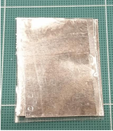
Figure 21: Seal Sample with Two Sides Taped
