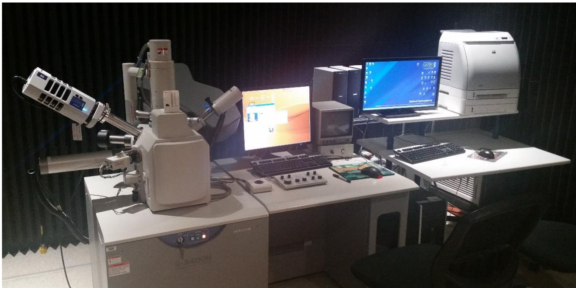
Figure 33: The Group of Machinery Utilizing the SEM and X-ray Detector
