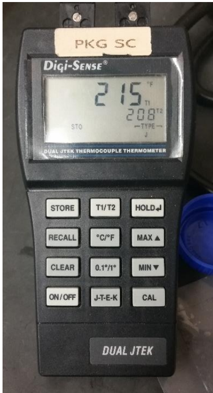
Figure 16: The Digi-Sense JTEK Thermocouple
