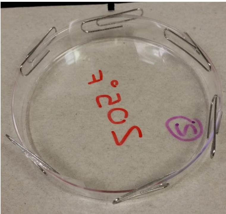
Figure 30: Seal Samples in a Petri Dish Soaking in NaOH
