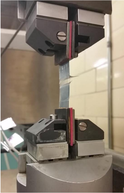
Figure 26: A Seal Sample While it is Being Pulled
