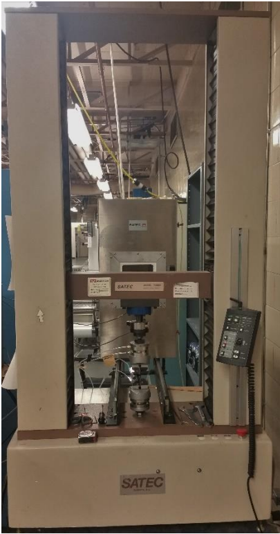
Figure 24: The Satec Instron when set to a 0.5" Jaw Opening
