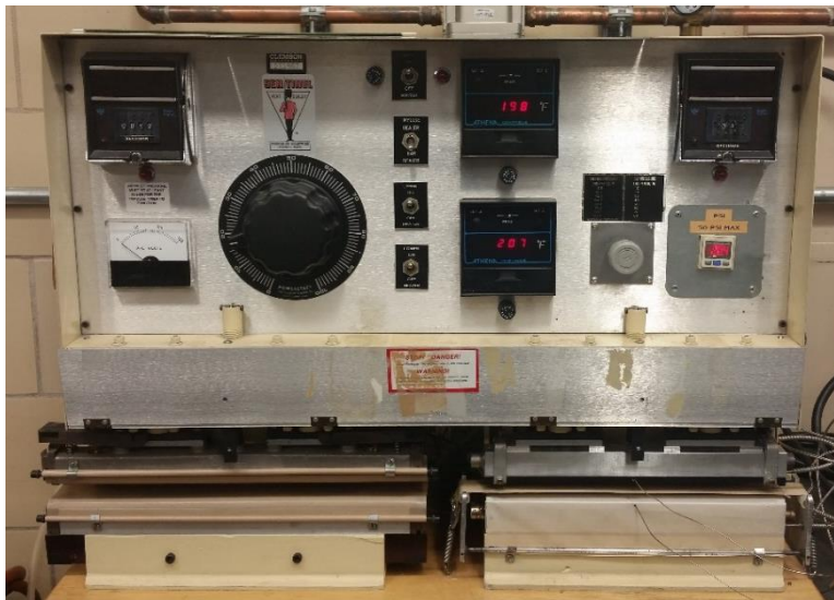
Figure 15: Sentinel Lab Scale Heat Sealer
