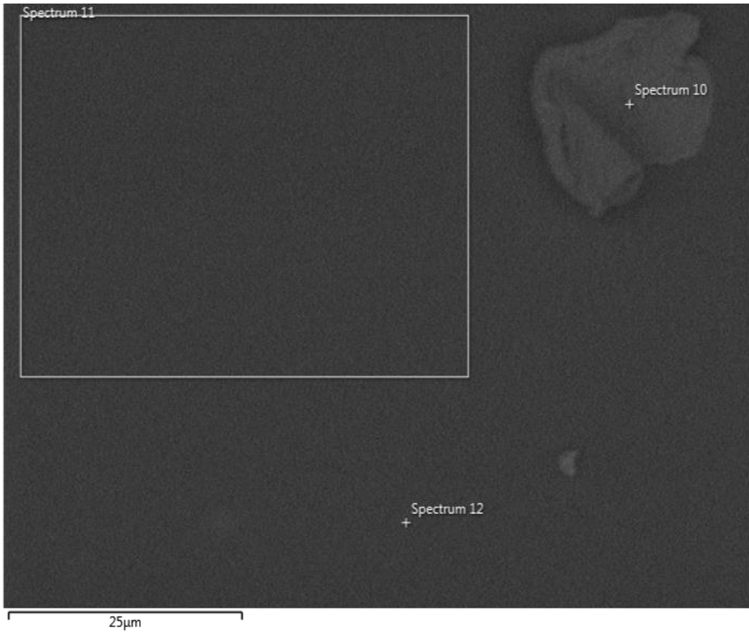
Figure 51: SEM Image of the Surface of DuPont Nucrel® 1202HC Not Exposed to NaOH
