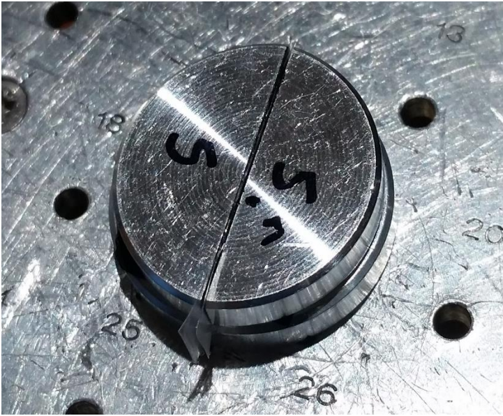
Figure 31: Polymer Sample Mounted Between Half Moon Discs for SEM
