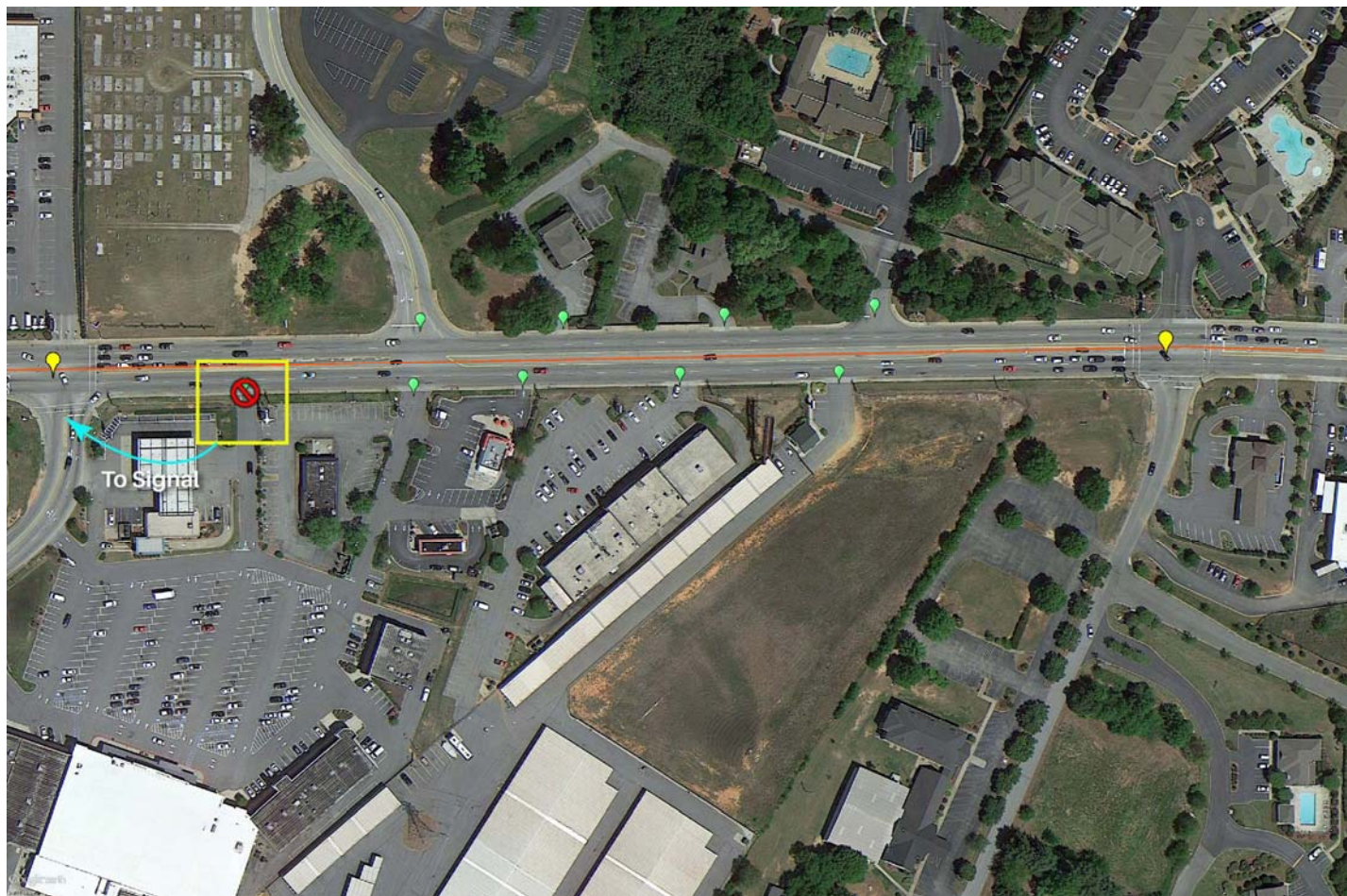
Figure 10d – Closing of Driveways within Minimum Acceptable Corner Clearance along Woodruff Road.
