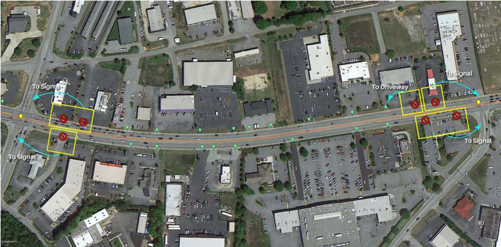
Figure 10c – Closing of Driveways within Minimum Acceptable Corner Clearance along Woodruff Road (cont. on following pages).
