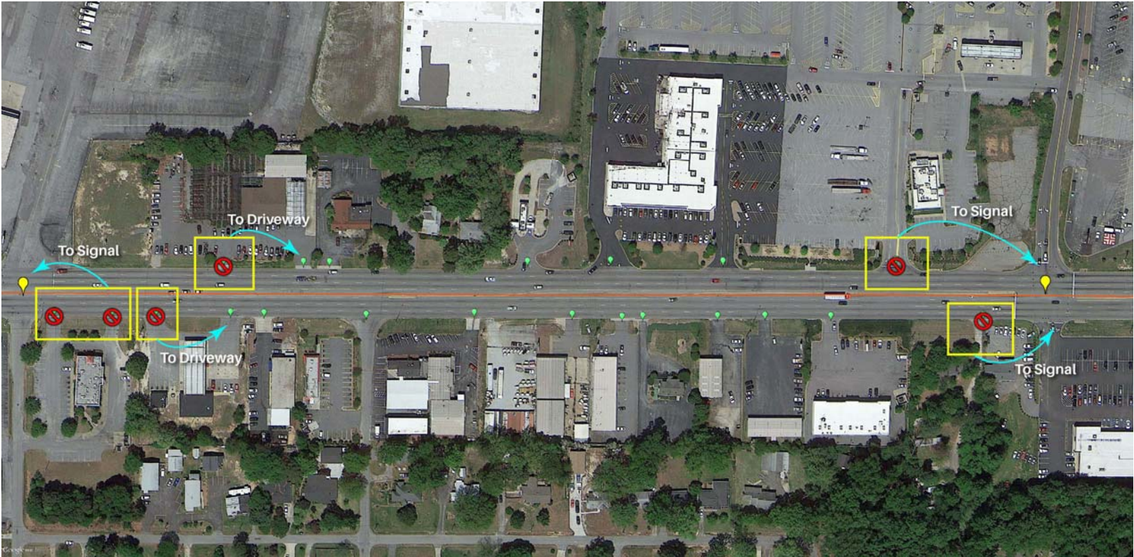
Figure 13c – Closing of Driveways within Minimum Acceptable Corner Clearance along Wade Hampton Blvd (cont. on following pages).
