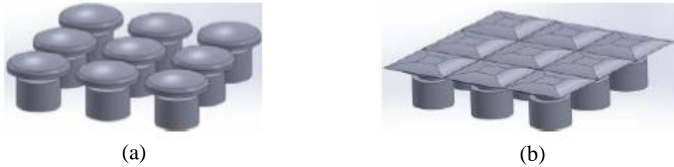
Figure 2.6: (a) Round pin heads, and (b) Square pin heads [33]
