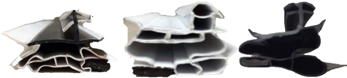
Figure 2.3: Cross sections of the investigated gaskets
