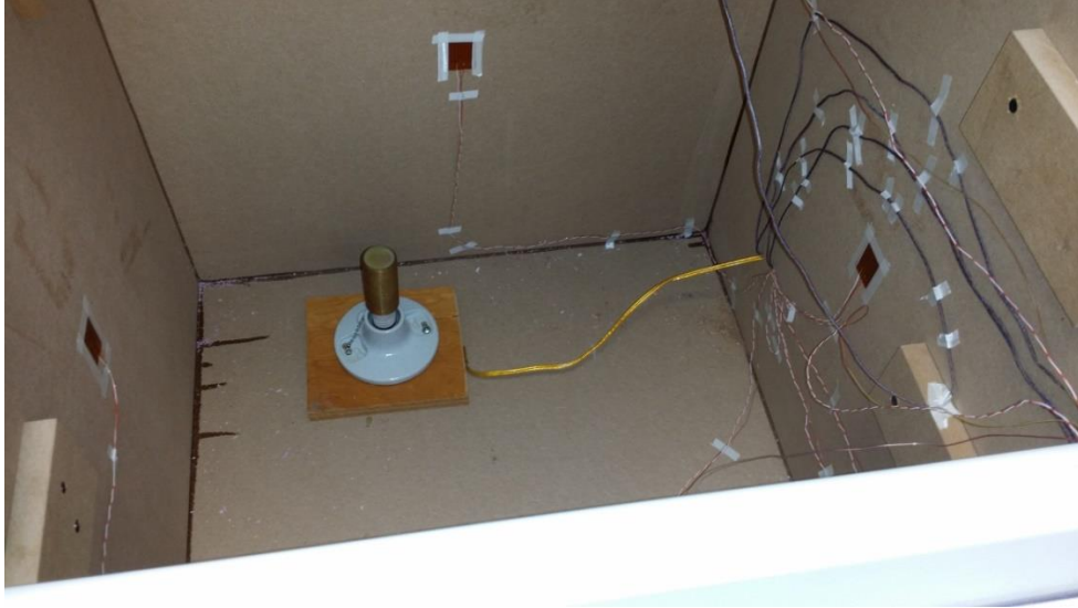
Figure 2.6: A view inside of the instrumented Blue Box (for experiments the heating element is centered within the box)
