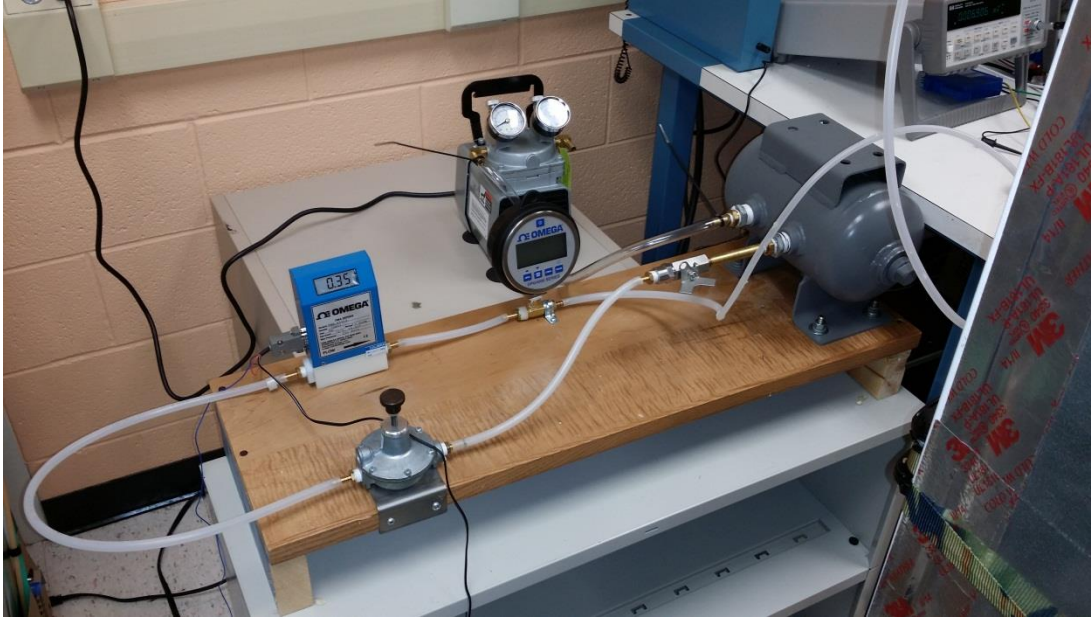
Figure 3.15: The experimental set up for pressurizing the refrigerator to find and seal the leakages.
