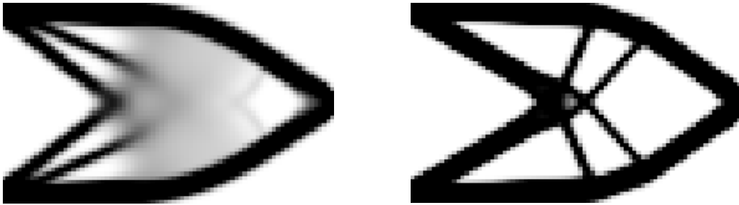
Figure 2.3. Example Solutions of SIMP Method with (left) p=1.5 and (right) p=3 [22]
