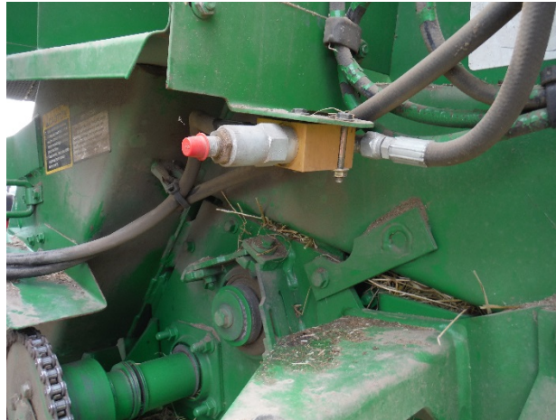
Figure 4.1. Where the pressure transducer was installed
