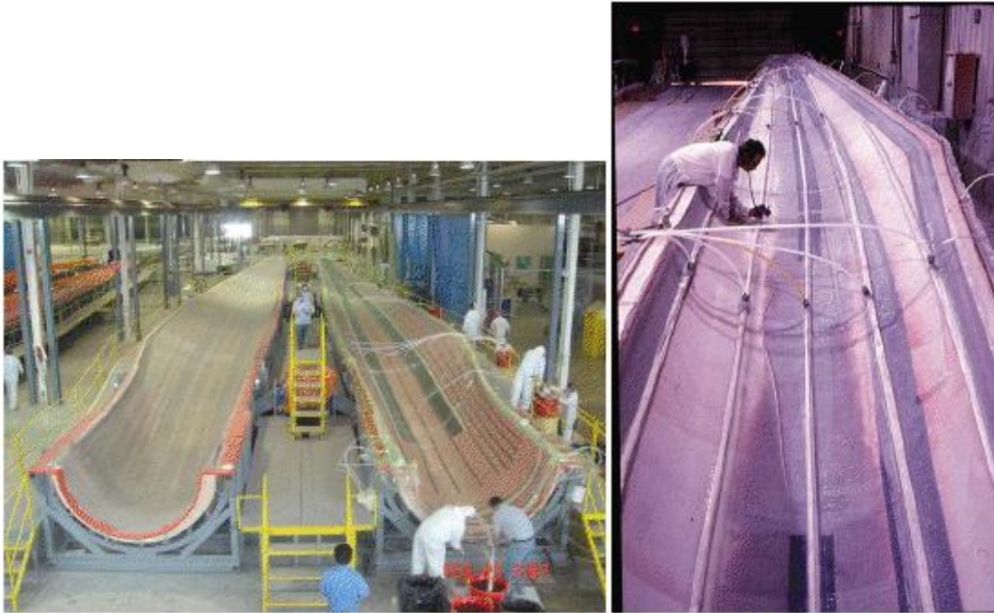
Figure 8: Set up of VARTM process rotor blade for wind turbine
