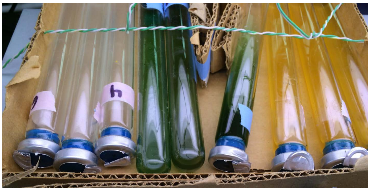
Picture Experimental Test Tubes at day 7 of RDX (5 \mu M) Degradation with Synechocystis in 10mM HEPES Buffer experiment. Left 3 test tubes (milky white) are light + RDX + 0.2mL Synechocystis capped in air; middle 3 test tubes (dark green) are light + RDX + 0.2mL Synechocystis anaerobic; right 3 test tubes (yellow, orange) are light + RDX + 0.2mL Synechocystis + AQDS capped in air.
