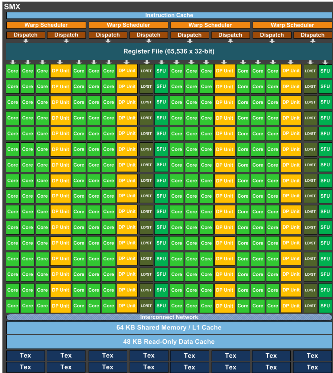
Figure 3.5: SMX in Kepler GK110 [5]
