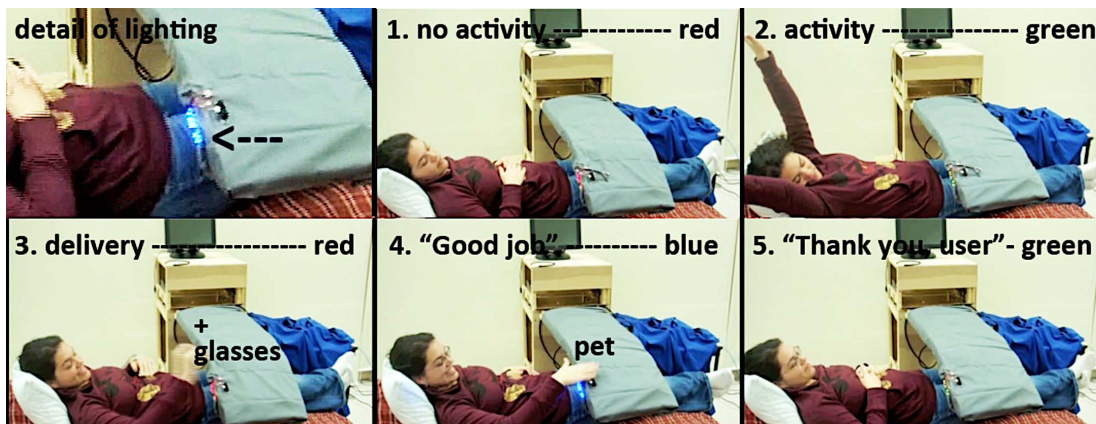
Figure 1.3: Stills from our video, showing our early-pilot development of ART and our NVC loop. The assistive robotic table is conversing to Jessica with lights (numbers and durations of blinks; color), and Jessica is reinforcing the table's actions by "petting" it.
