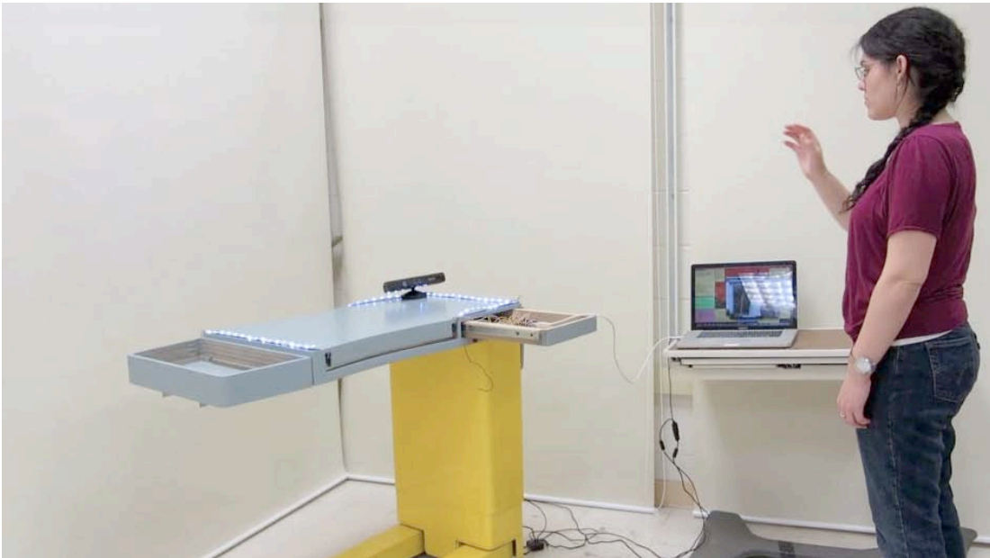
Figure 3.2: Presented is the NVC platform evaluation set-up for Phase II and III. Push buttons and a Microsoft Kinect ® were used to actuate each NVC action and sounds were played through an adjacent computer.
