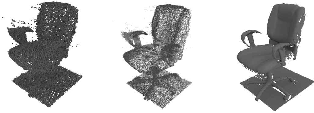
Figure 5.2: A reconstruction of a typical office chair. The chair was reconstructed using a 3D occupancy grid (left and middle) and a TSDF (right). The left occupancy grid and the TSDF reconstructions had a resolution of 1cm while the middle occupancy grid had a resolution of 5 mm. It is clear that the TSDF provides a more detailed reconstruction and does not contain as much noise as the 3D occupancy grid. When the left occupancy grid and the TSDF representations were stored in an octree the 3D occupancy grid consumed 1.5 MB of memory and the TSDF consumed 3.6 MB of memory. The middle occupancy grid consumed 2.96 MB. Without the use of an octree the left 3D occupancy grid would have required 12.5 MB of memory to store and the TSDF would have required 402.65 MB of memory to store when using volumes that were 512 x 384 x 512 voxels in size. The octree provided 8.3 : 1 compression ratio for the 3D occupancy grid and a 111.85 : 1 compression ratio for the TSDF.
