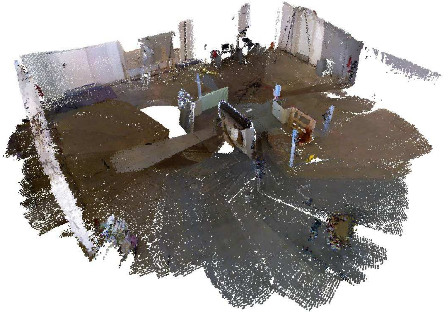
3D Occupancy Grid, 50mm resolution, Stored in an octree with 497 MB of memory.
