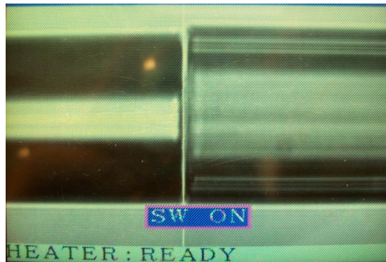
Fig. B.1. MMF and capillary tube alignment under the view of fusion splicer monitor. Left: MMF, right: capillary tube.
