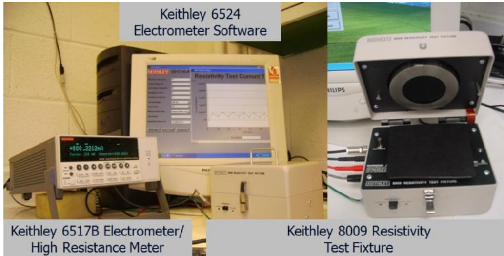
Figure B.6. Keithley 6517B High Resistance Meter and Keithley 8009 Resistivity Test Fixture.
