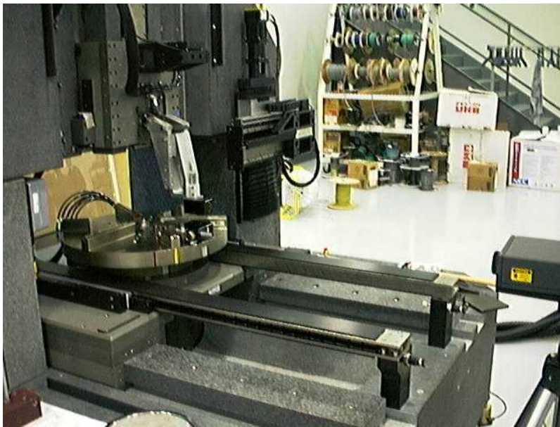
Figure 2: Universal Measuring Machine
