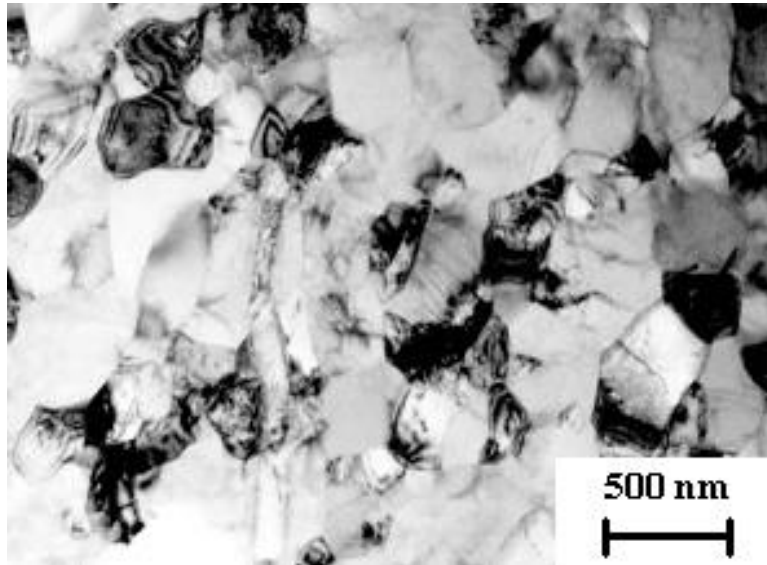
Figure 15: Microstructure of the ECAP material [1].
