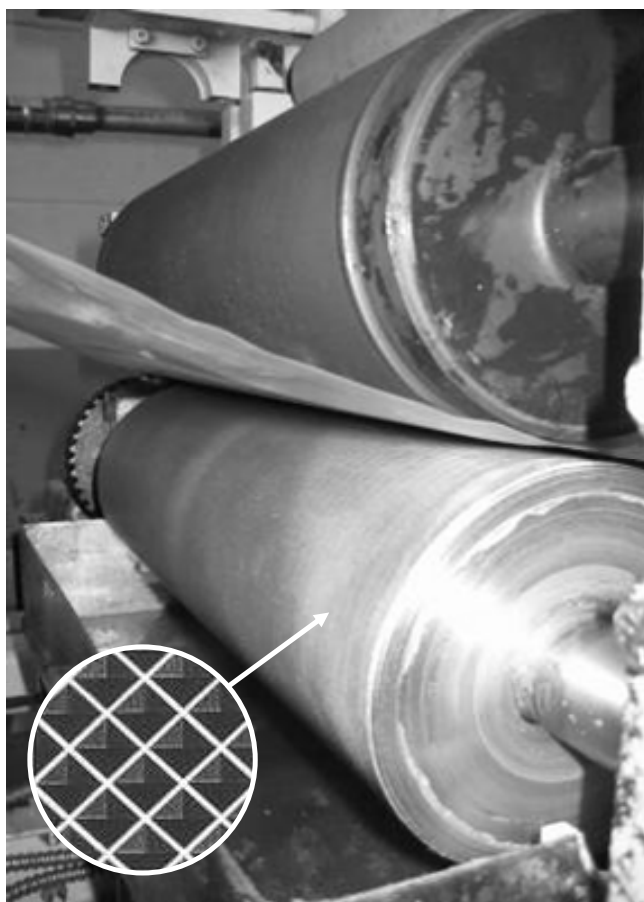
Figure 11: Sample for the surface (dpi) of a gravure roll
