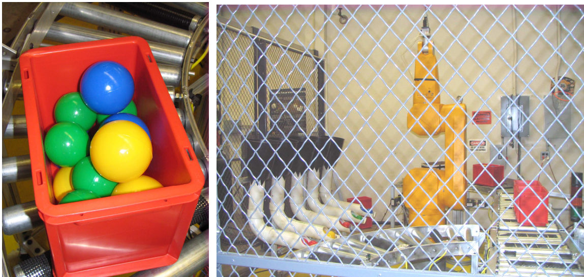
Figure 2.10: Shipping container with ball order fulfilled and complete sorting system
