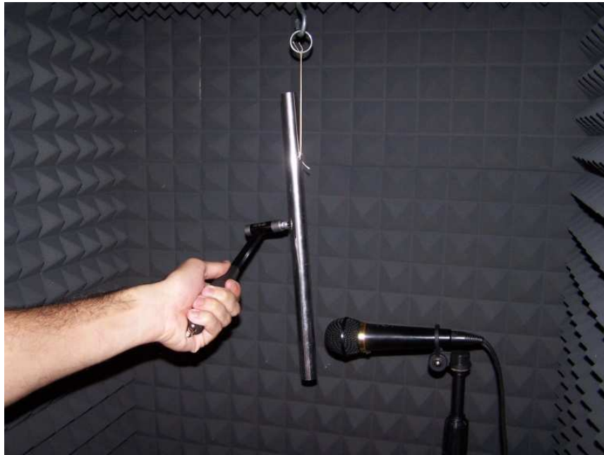
Figure 3.2 Set up for acoustic experiment
