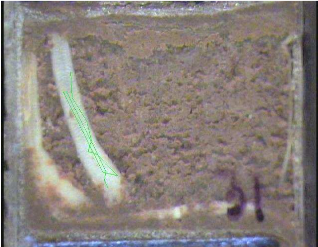
Figure 2.8: This image show the network doubling back on itself if the energy function does not have a term to prevent the line segments from doubling back on network.
