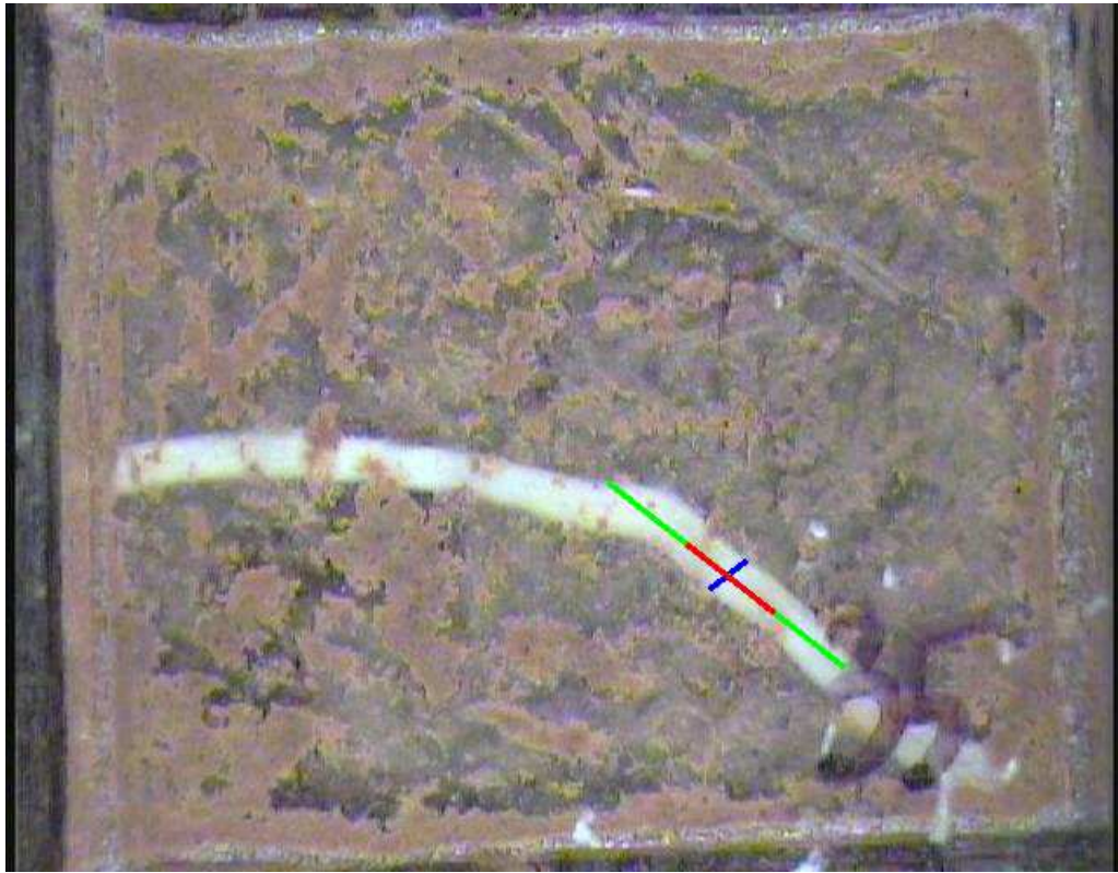
Figure 2.6: This image show how the aspect ratio is calculated. The aspect ratio is the length (in pixels) of green line to the length (in pixels) of blue line.
