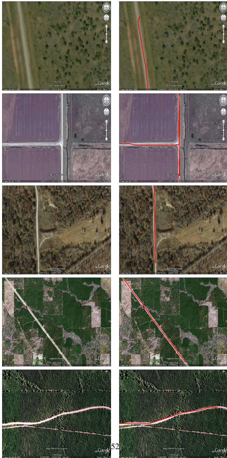
Figure 6.1: Left image: the original image. Right image: the detected roads.
