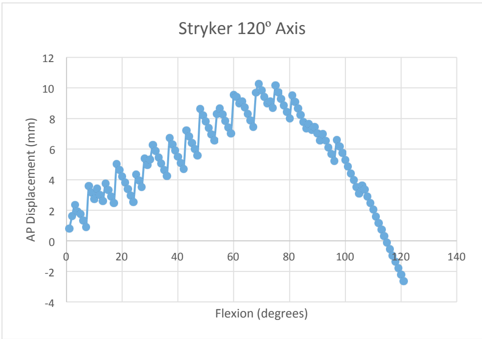
Figure B.5: A/P displacement of Stryker Triathlon® at ideal axes for 60 and 120 degrees flexion.
