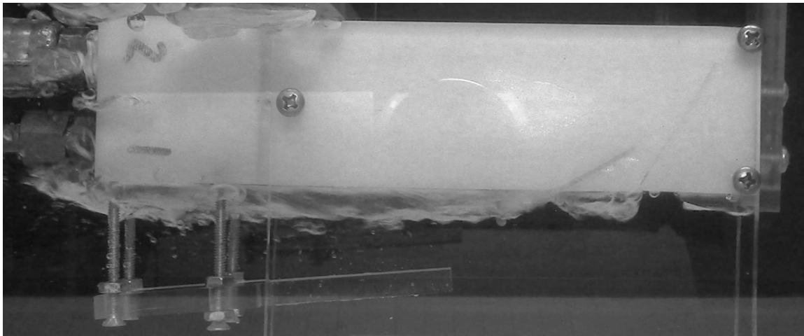
Figure 21. Concurrent steam and CA ventilation showing entrainment of CA by the steam vent; low ventilation ratio. Notice continuation of continuous cavity downstream of steam vent with large scale bubbles breaking from rear of cavity.
