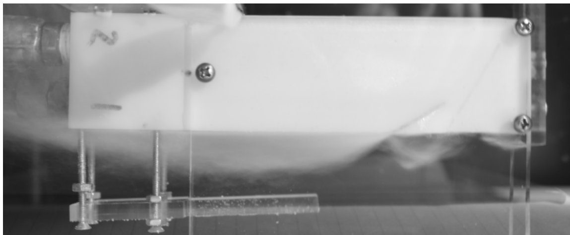
Figure 22. Long exposure photograph of concurrent steam and CA ventilation showing entrainment of CA by the steam vent; moderate ventilation ratio. No continuous cavity remains aft of steam vent but rather a frothy mass of bubbles.
