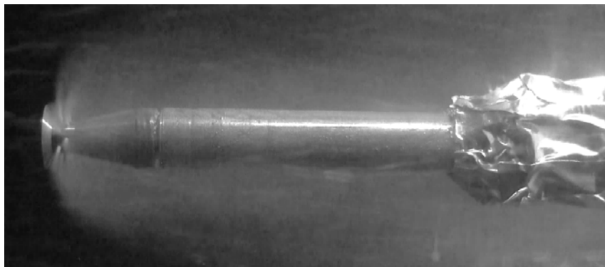
Figure 31. Steam only ventilation at 8 CFM for disc cavitator.
