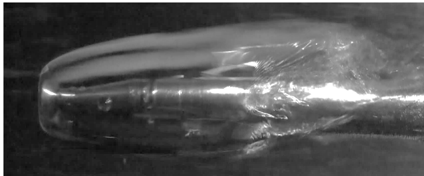
Figure 27. Disc cavitator for air ventilation at 0.01 CFM. Clear and smooth cavity can be seen. Similar cavity shapes were seen for ventilation at 0.1 CFM and for film cavitator.
