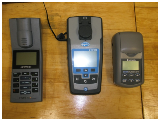
Figure 3.1. Selected nephelometers. From left to right GW, Hach 1, and LaMotte.
