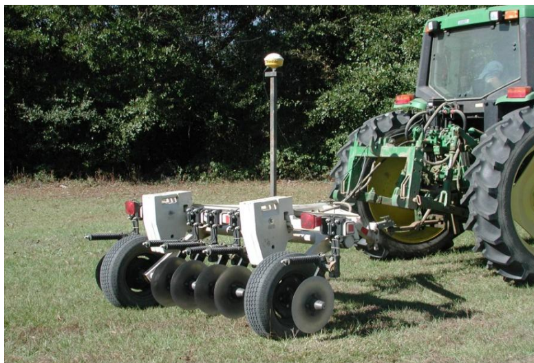
Figure 1.1. Geo-Referenced Veris 3100 Soil EC Meter.
