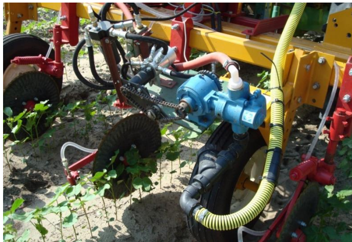
Figure 2.4. The side-dress Nitrogen applicator with retrofitted Rawson controller.
