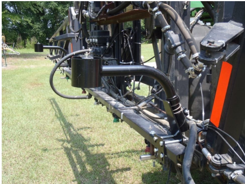
Figure 2.12. NORAC ultra-sonic height sensors.
