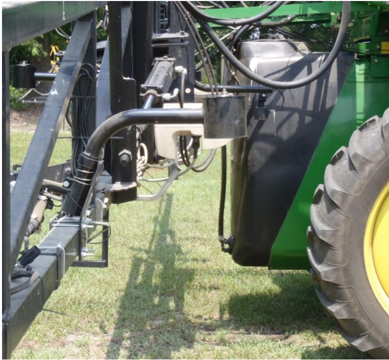
Figure 2.7. UC4+ Ultrasonic Sensors and GreenSeekers®.
