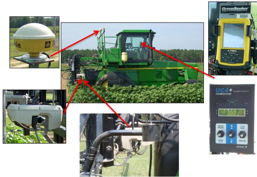
Figure 2.6. John Deere 6700 with NTech GreenSeeker® RT-200 system.
