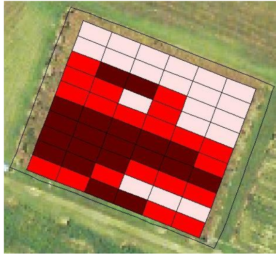
Figure 1.8. . Average EC Plots in the Irrigated test Field (2007).
