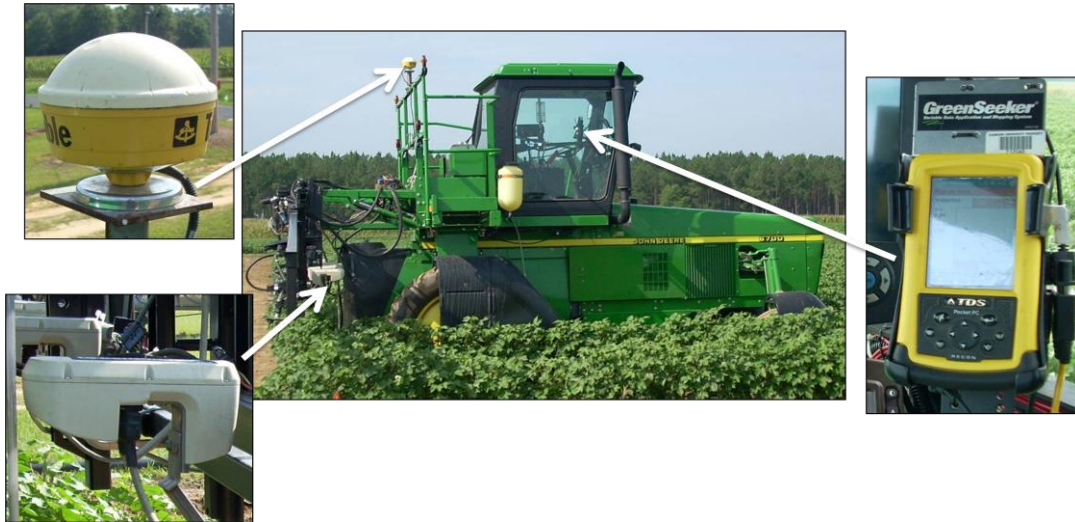
Figure 1.4. Sprayer Mounted GreenSeeker® RT-200 System.
