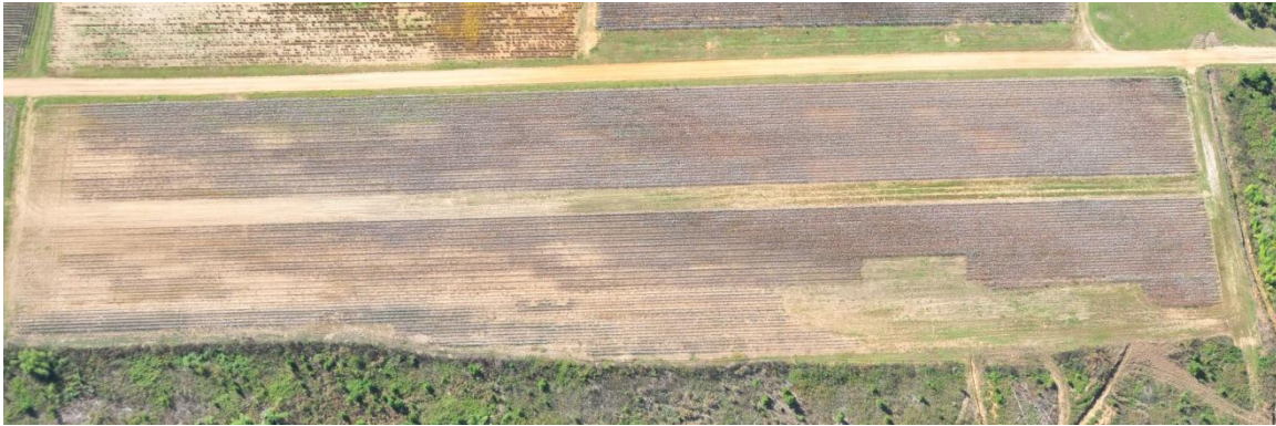
Figure 2.5. Aerial photo of uneven plots caused by GPS and software errors.
