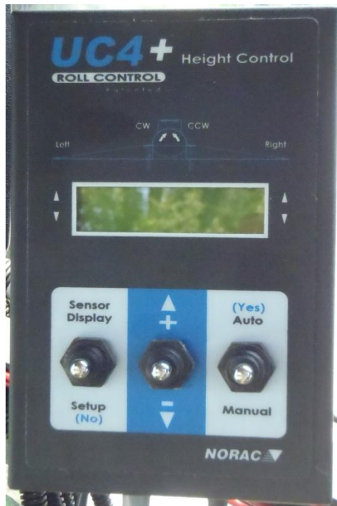
Figure 2.8. UC4+ Height Controller.
