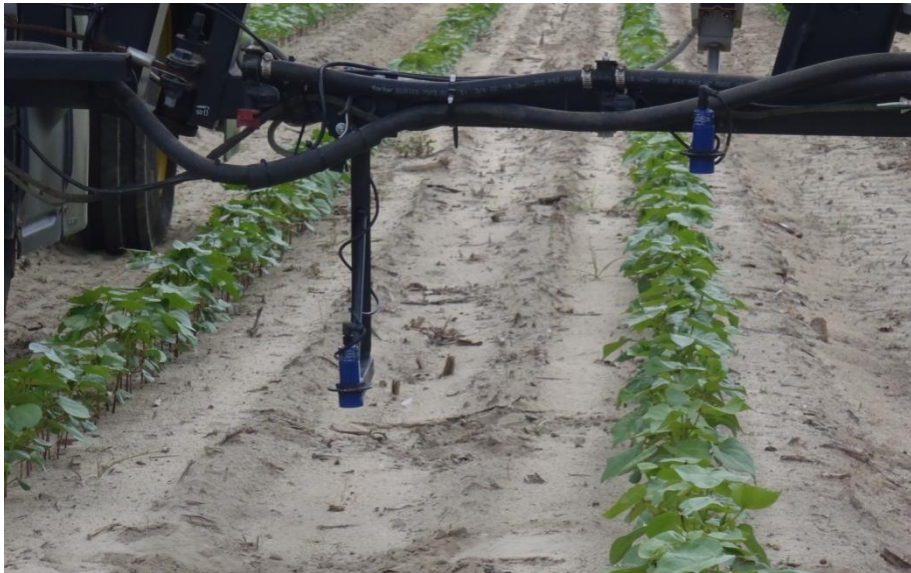
Figure 2.11. Mounting locations of the HP sensors on the sprayer boom.
