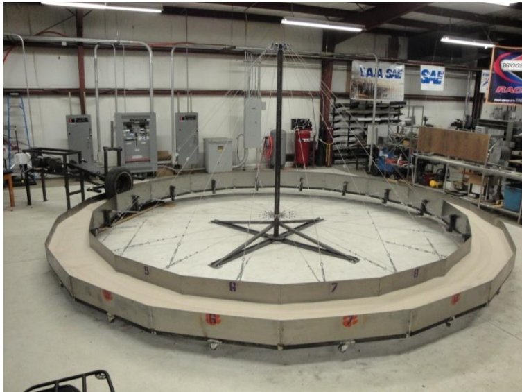
Figure 1.2: Lunar wheel endurance testing system [21].
