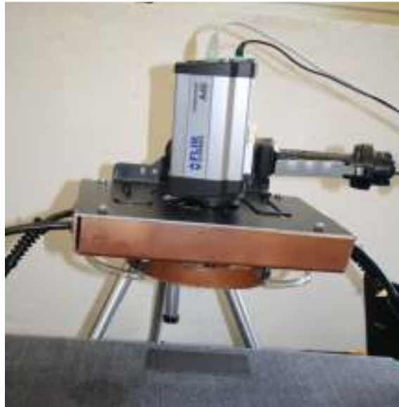
Figure 4.14 Experimental Setup for Thermal Imaging with Flash Light as Heat Source.
