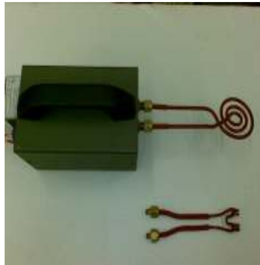
Figure 1.9 (b) Induction Coils [6].
