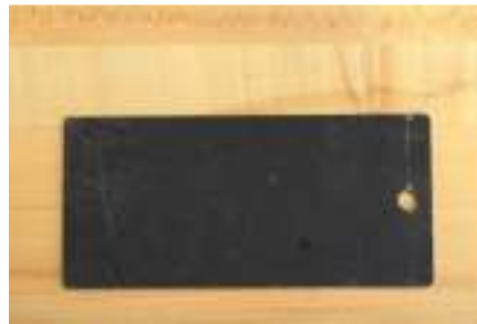
Figure 4.11 Galvanized Steel Plates With Adhesive Spots.
