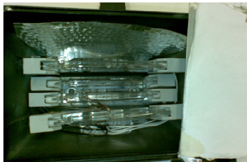
Figure 1.7 Halogen Lamps used as Heating Source [6].
