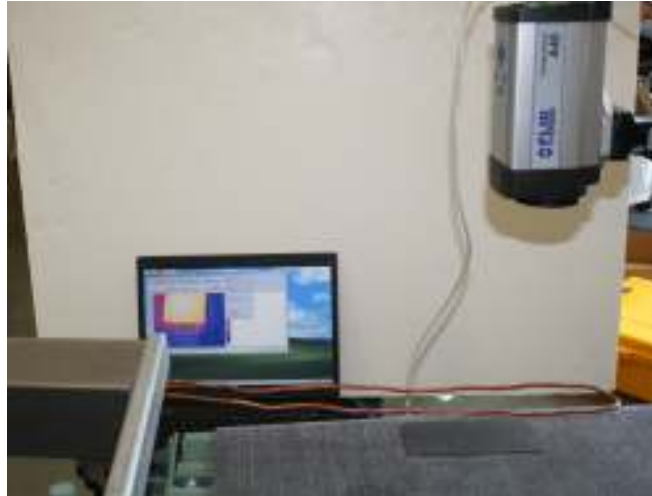
Figure 4.12 Experimental Setup for Thermal Imaging with Induction Coil as Heat Source.
