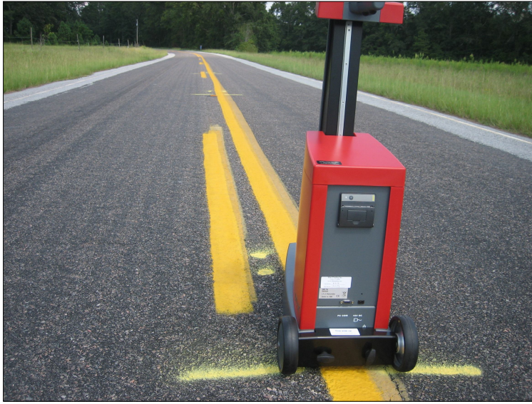
Figure 3.4: Retroreflectometer Collecting Data
