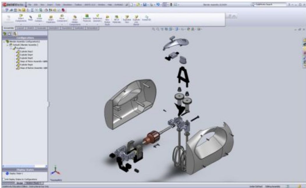
Exploded View of Durabrand Blender
