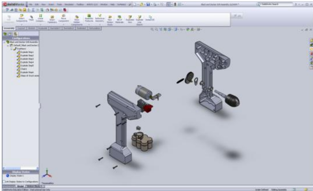
Exploded View of Black and Decker Drill
