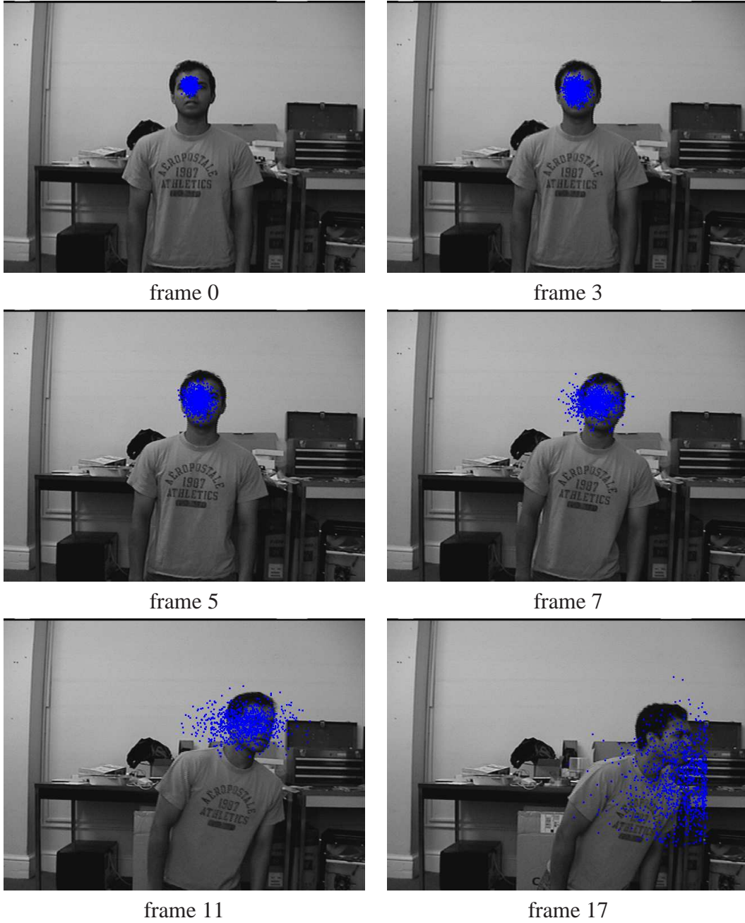
Figure 6.1: In the images, the blue dots show the particles. These images show the behavior of the particles in absence of resampling.
