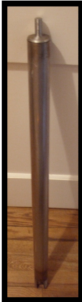
Figure 2.12: The reference rod is a hollow cylinder with two end pieces used to attach to the top anchor and the top of the strain bar.
