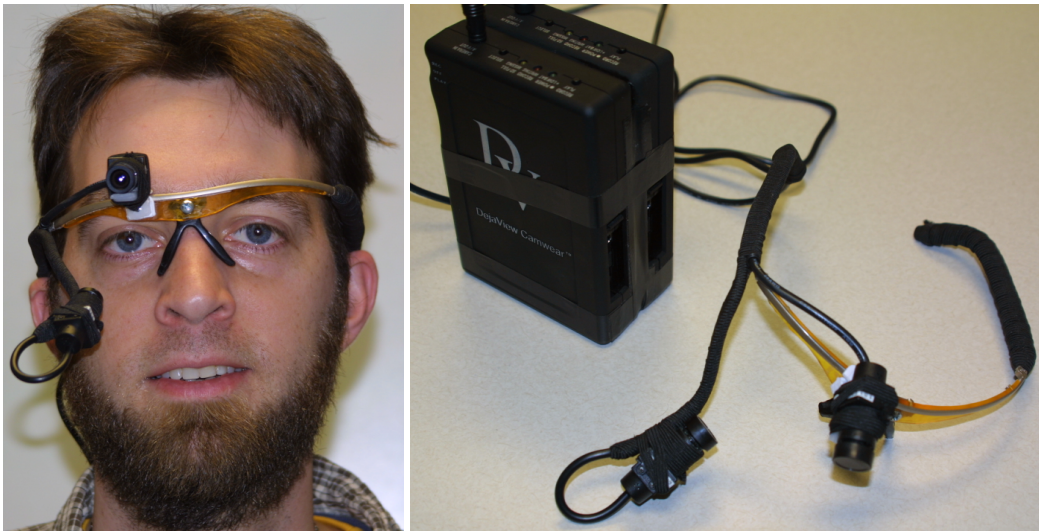
Figure 1.1: Our “DIY” wearable eye tracker from relatively inexpensive (~$700) off-the-shelf components.
