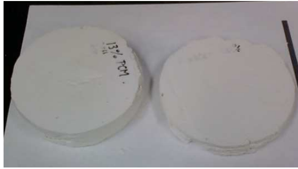
Figure 3.1. Cylindrical samples made of PCM mixed in plaster
