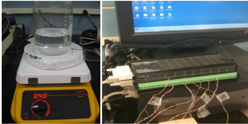
Figure 4.2. Thermal conductivity experimental setup (left) and data acquisition system (right)
