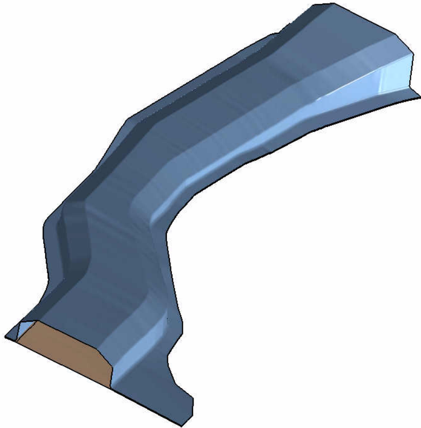
Figure 6-5 Semi hexagonal shape of the Frontal longitudinal rail
