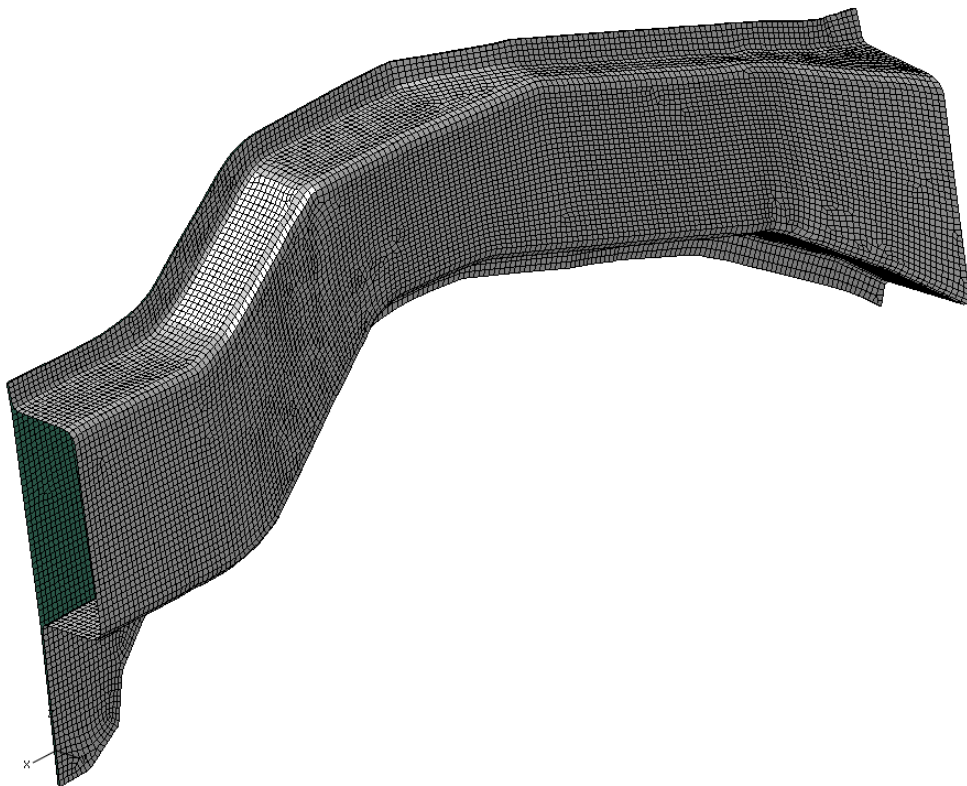
Figure 5-13 Mesh on frontal longitudinal rail created using HYPERMESH
