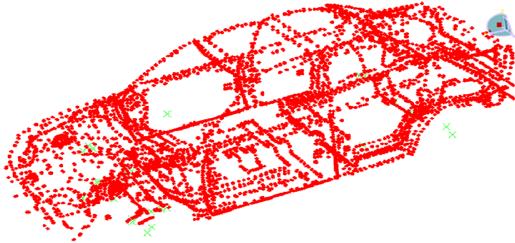
Figure 5-2 Single node-to-node rigid spot welds in the entire FEA model of Dodge Neon
