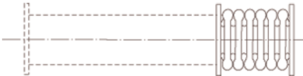
Figure 1-2 Axial collapse mode for closed section tube [5]
