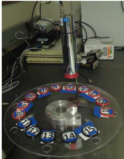
Figure 5.7: Rotary Table Setup for Gamma-ray Attenuation Procedures for Gamma-ray Attenuation and External Dosimetry Lab
