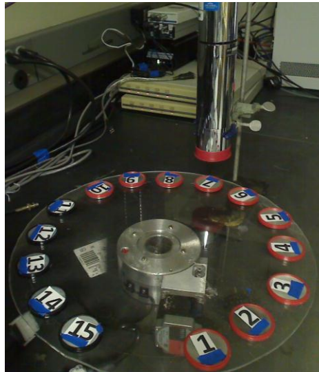
Figure F.3: Rotary Table Setup for Gamma-ray Attenuation Procedures
