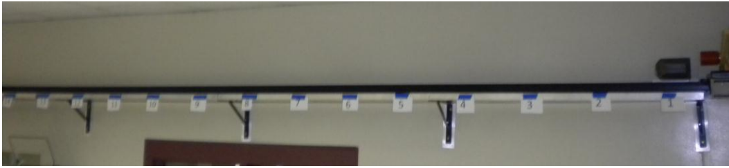
Figure 5.8: BiSlide™ Setup for External Dosimetry Procedures for Gamma-ray Attenuation and External Dosimetry Lab
