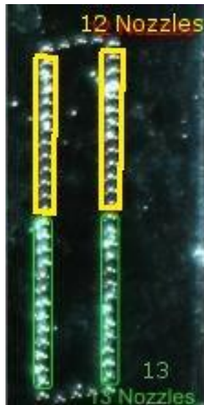
Figure 2-16 Close-up of HP26 Quadrants at 10x Magnification
