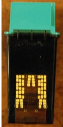
Figure 2-21 Flex Circuit of the HP 26 Cartridge
