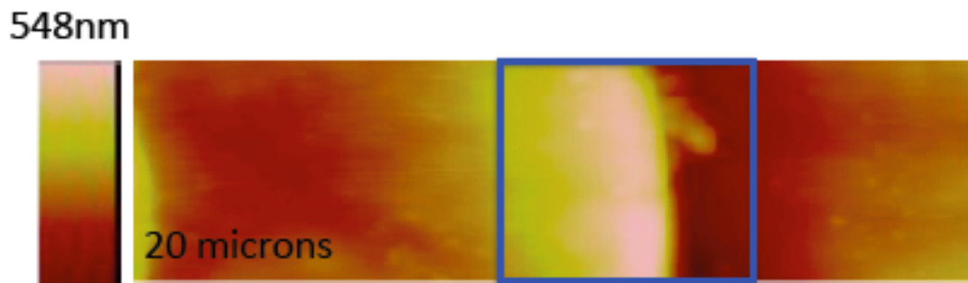
Figure 2.10: An example of AFM being used to develop a topographical image of a sample surface. This particular sample is a wool fiber, including a scale edge, indicated by the box.
