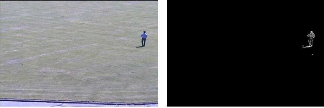
Figure 5.2: The figure shows an example image of a person along with the respective strength map obtained using linear combinations of RGB. Using such strength maps obtained in each frame, the objects are being tracked.
