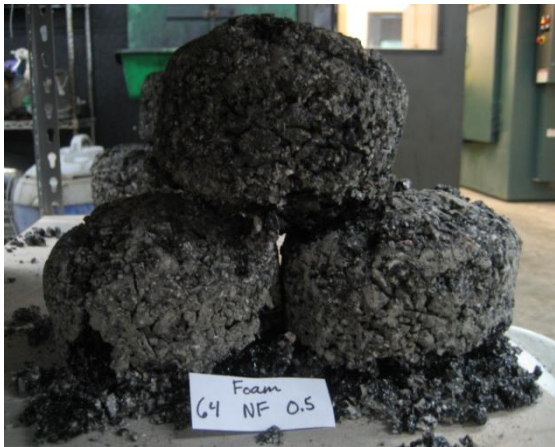
Figure E.14: Unaged vs. PG 64-22 Foam NF +0.5% Note: * denotes that sample collapsed or deformed during aging.
