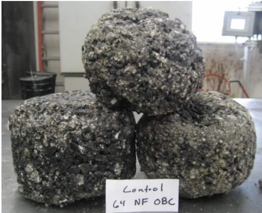
Figure E.9: Unaged vs. Aged of PG 64-22 Control NF OBC Note: * denotes that sample collapsed or deformed during aging.
