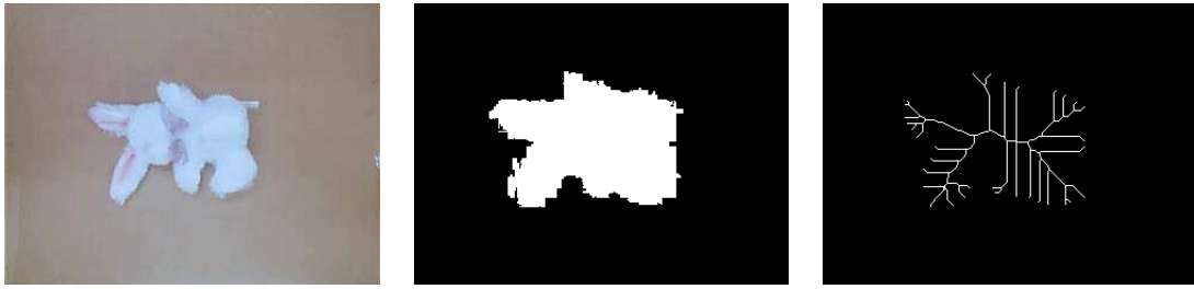
Figure 3.3: LEFT: The original object. MIDDLE: The isolated object to be classified. RIGHT: The skeleton of the object.
