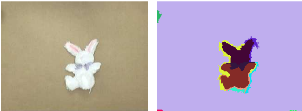
Figure 2.2: LEFT: An image taken in our lab. RIGHT: The results of applying the graph-based segmentation algorithm. Despite the over-segmentation, the results provide a sufficient representation for grasping the object.
