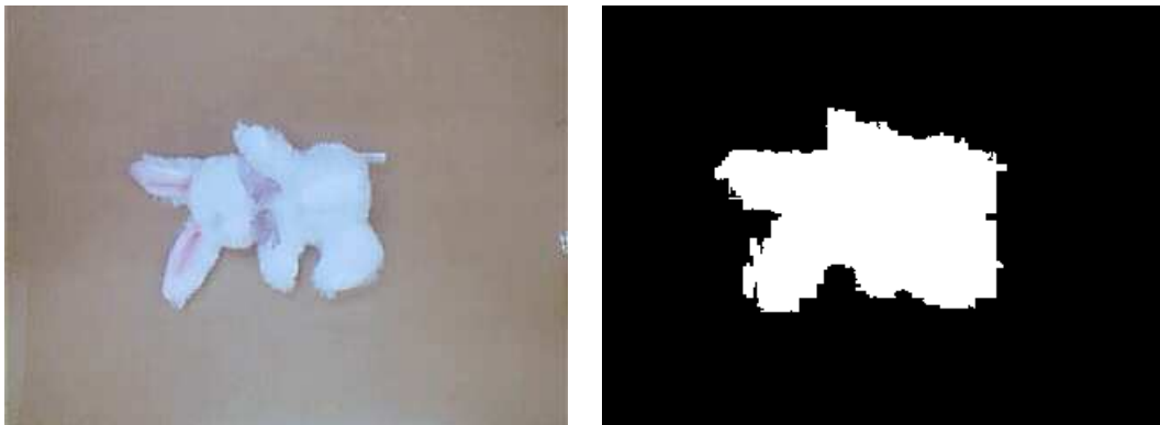
Figure 3.2: LEFT: The isolated object to be classified. RIGHT: The binary mask of the object used in constructing its color histogram model.
