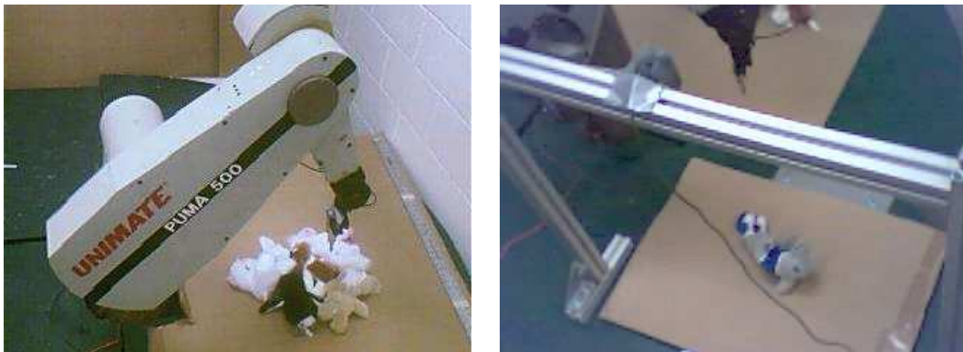
Figure 1.1: The proposed setting for manipulation-guided sensing. Left: A robotic arm interacts with a pile of unknown objects (stuffed animals) to segment the individual items one at a time. An overhead stereo pair of cameras (Logitech QuickCam Pro webcams) is not shown. Right: The system then learns about each object’s characteristics by automatically isolating it from the pile and interacting with it. A third overhead camera is used for sensing the isolated object.
