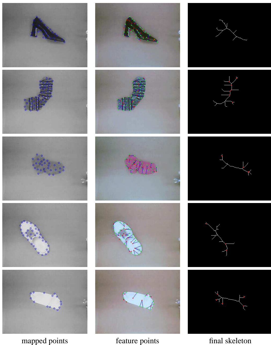
Figure 4.18: Continuing the same experiment from Figure 4.17. From left to right: The feature points gathered from the isolated object, the image after mapping the feature points to the intersections points, and the final skeleton with revolute joints labeled. Time flows from top to bottom, showing the progress as each individual object is examined.
