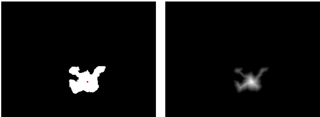
Figure 2.4: LEFT: The binary region associated with an object. The grasp point (red dot in the center) is the location that maximizes the chamfer distance. RIGHT: The chamfer distance of each interior point to the object boundary.
