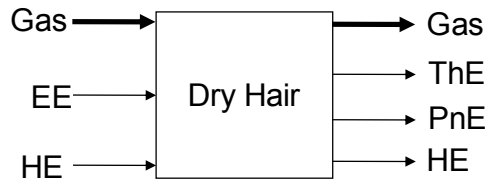
Figure 13: Black-box function structure for the hair dryer product
