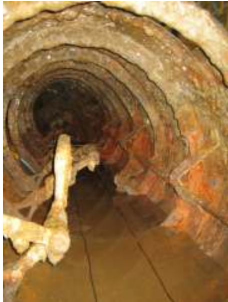
Figure 5.1. The corrosion in the H.L Hunley submarine (Photo courtesy of the Friends of the Hunley)
