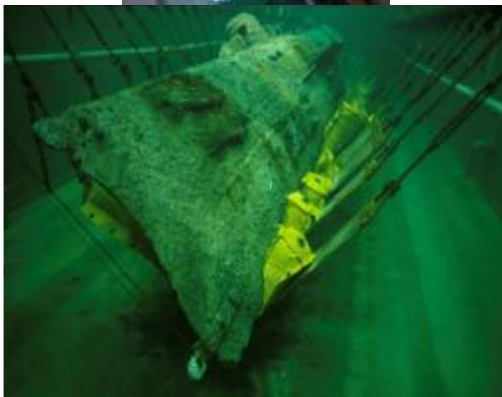
Figure 1.2. H.L. Hunley, cushions and sling system in conservation tank (Photo courtesy of the Friends of the Hunley)
