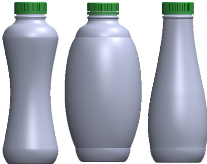
Figure 14. Bottles created in Solidworks.
