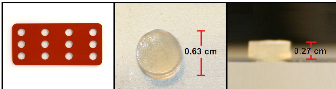
Figure 7: Silicone Isolator (Left), Hydrated 5% TEGDA/30% AEMA Hydrogel from Study B diameter (Center) and thickness (Right) dimensions.
