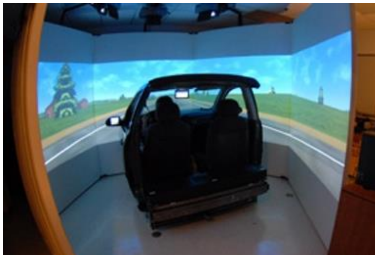
Figure 1. The room used during data collection with driving simulator pictured in the middle.
