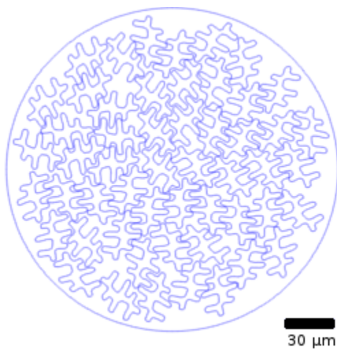
Figure 1.2: The column wall is represented by a polygon which approximates a circle. The disjoint fiber-polygons are arranged in a similar way as the fibers in Figure 1.1. The inner column wall has a diameter of 215 \mu m . The polygon-fibers have a diameter, cf. Definition 2.2.2, of 30 \mu m . The data for this diagram is from [7].
