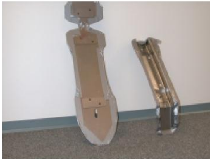
Figure 3-6 A panel made using Patch TWB and Stamping [29]
