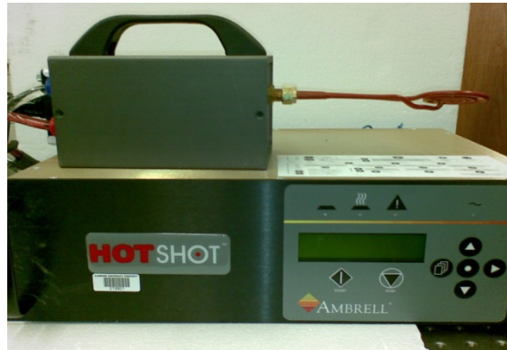
Figure 5.3.3: Induction Heating Source
