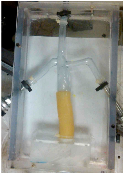
Figure 16: Transparent, rigid TCPC model mounted within an open box
