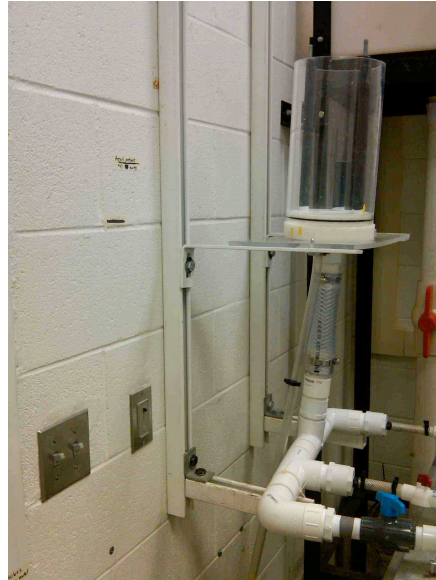
Figure 4: The systemic arterial pressure head tank of adjustable height
