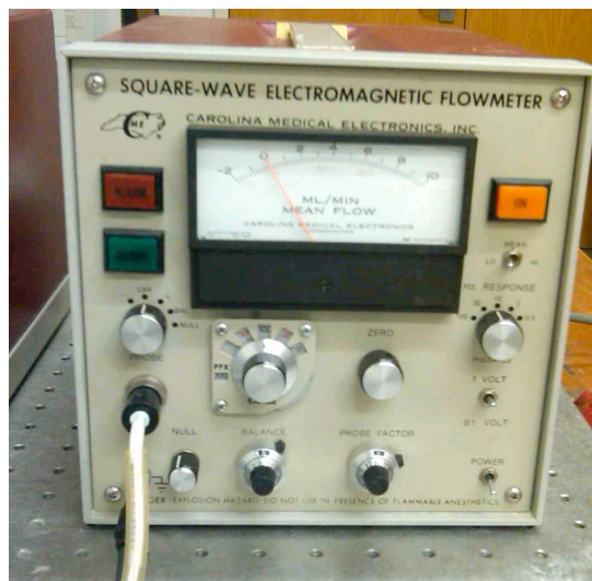
Figure 23: FM501 Electromagnetic flow meter
