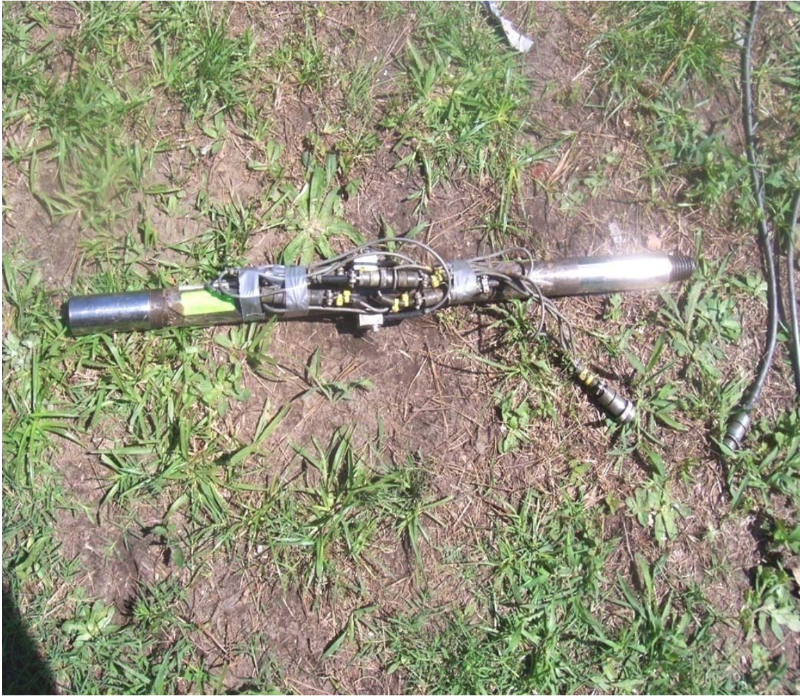
Figure 2.8 SPT energy measuring equipment that was attached to the rods.
