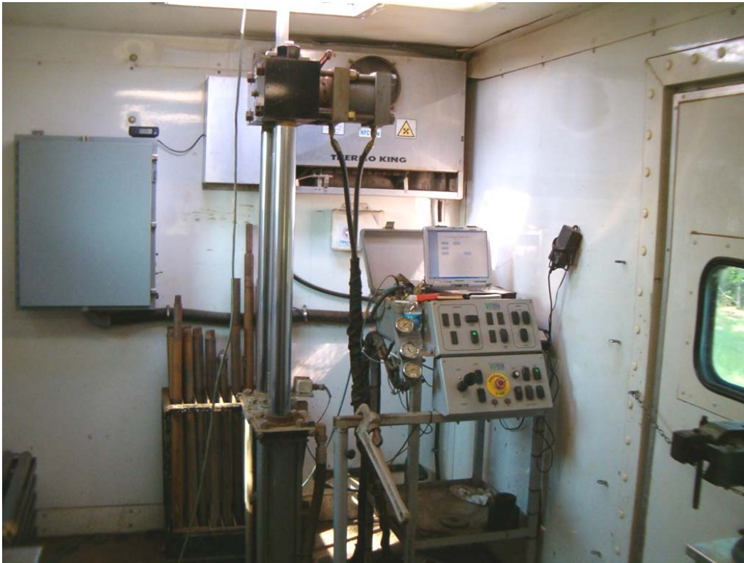
Figure 2.2 Data acquisition station and hydraulic assembly inside the cone truck.
