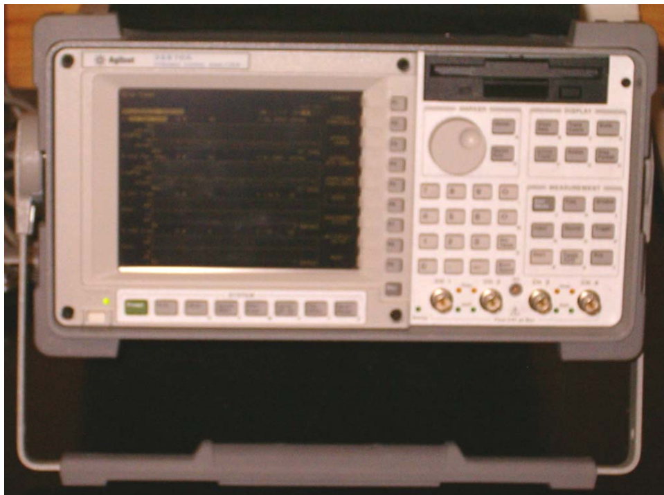
Figure 2.11 Agilent Technologies dynamic signal analyzer used for collecting and analyzing seismic crosshole test data.
