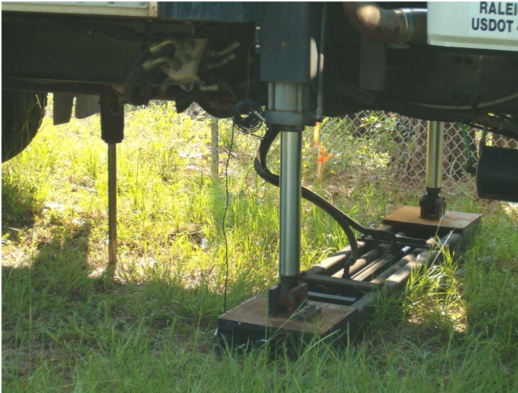
Figure 2.1 SCPTu truck rig's front leveling jack, which also serves as the source of the seismic energy for true interval velocity measurements.
