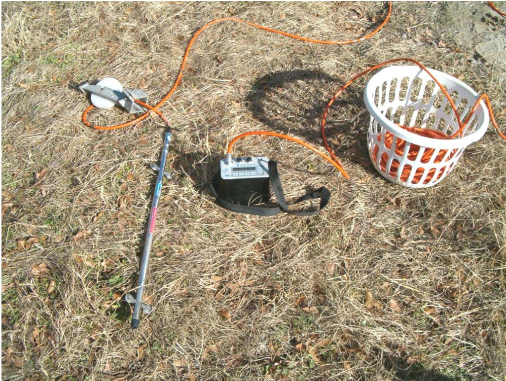
Figure 2.16 Digitilt Slope Inclinerometer system manufactured by DGSi.
