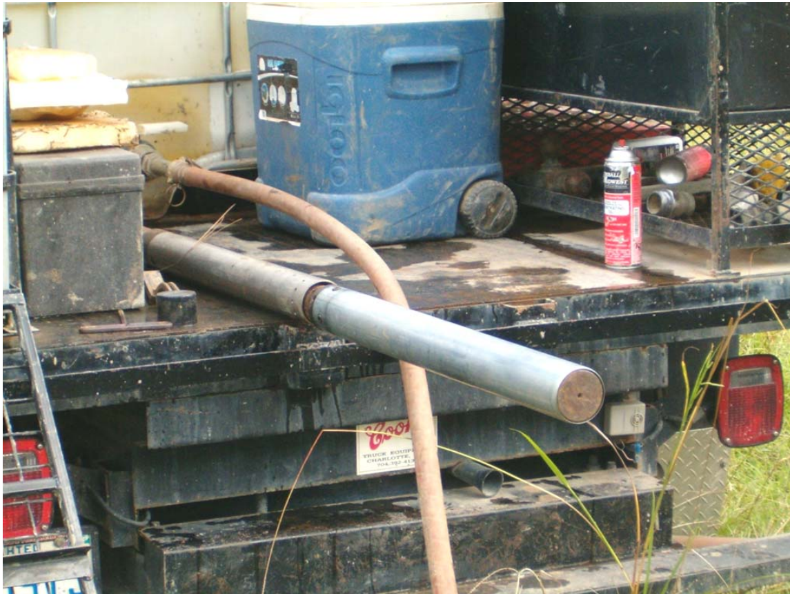
Figure 2.7 Osterberg sampler used at the Walterboro Rest Ponds site.
