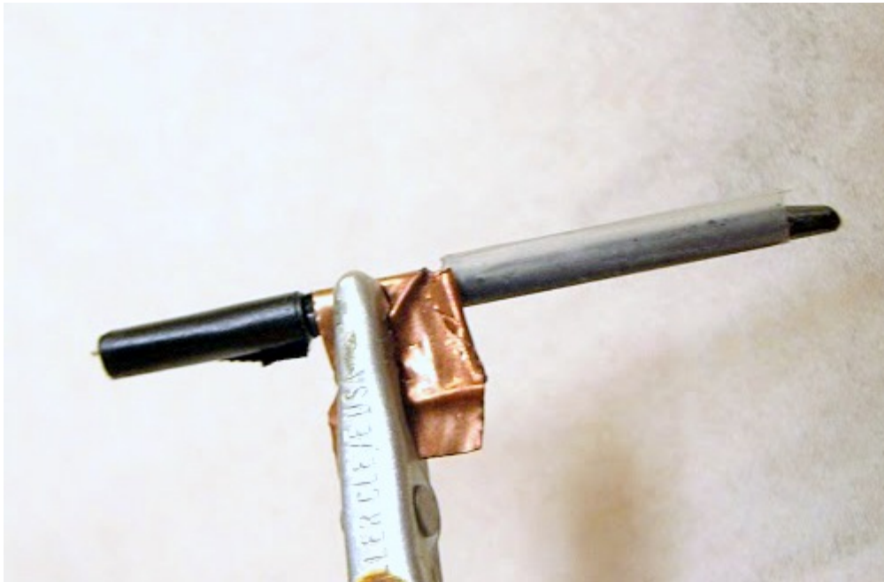
Fig. 5.9. Graphite probe attached to an alligator clip.
