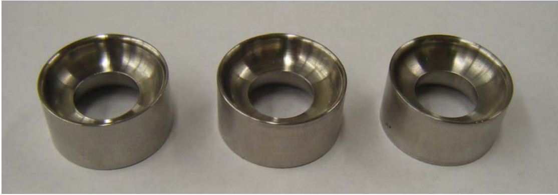
Figure 3.2: Diodes, from left to right: 60^\circ , 75^\circ , and 90^\circ\alpha .
