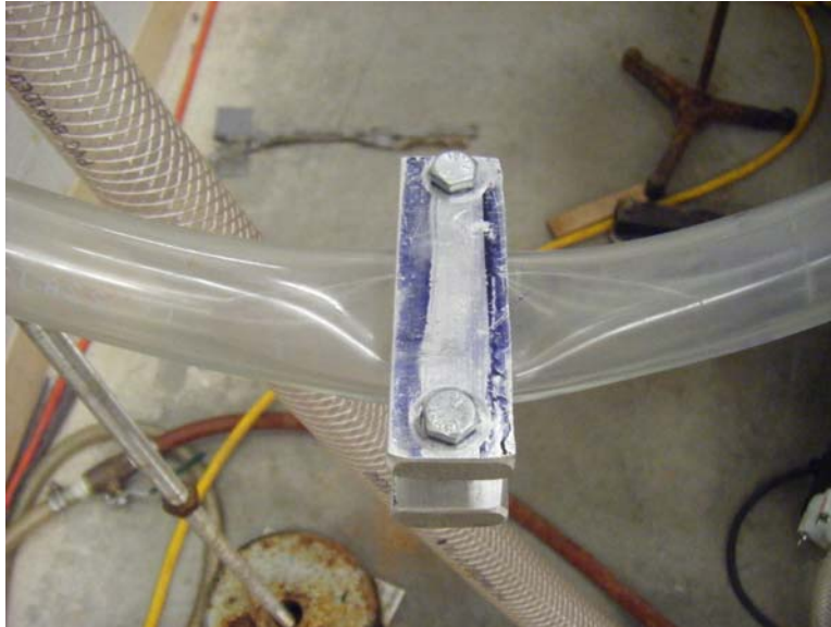
Figure 3.13: Hose clamp used as a resistance element.
